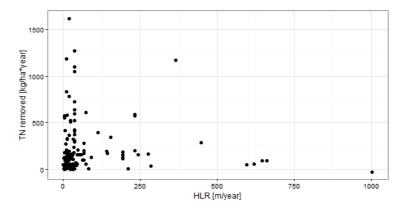
Figure 1: Relationship between total nitrogen (TN) removal and hydraulic loading rates (HLR) (n=146)
