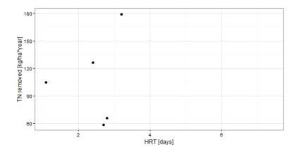
Figure 2: Relationship between total nitrogen removal and hydraulic retention time (HRT) (n=5 → due to incomplete variable HRT)
