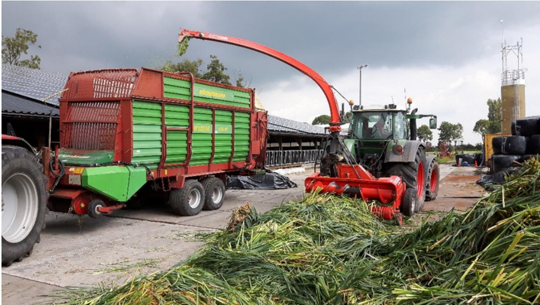
Fig.: Chopping Typha with a maize chopping device for ensilaging
