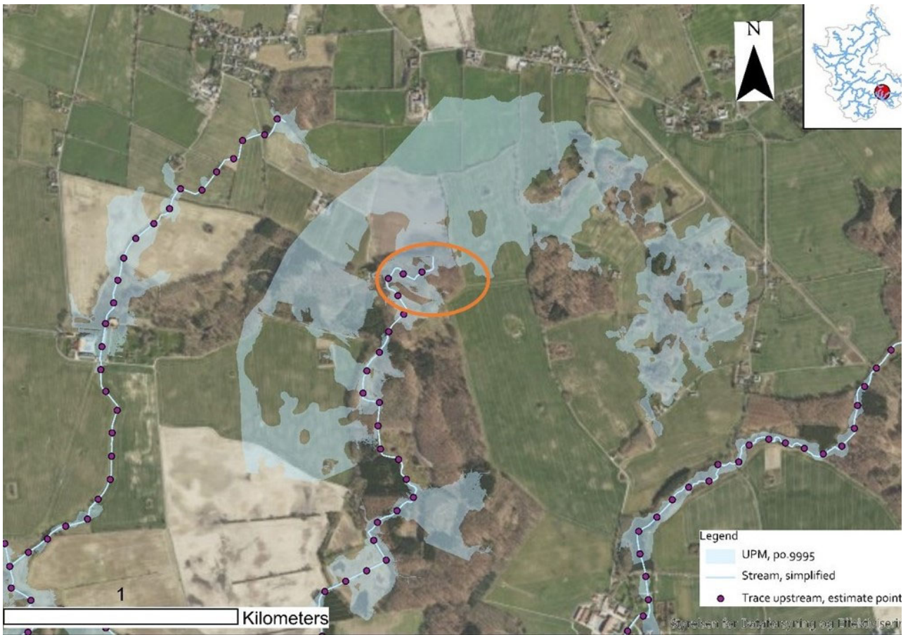
Figure 3.1.1.3. Map enlargement showing areas where flooding is overestimated. The stream in the centre is wrongly delineated over a local top in the landscape (wrong delineation in the orange marking). This results in an overestimated raise in waterlevel causing a large spillover upstream the stream course.
