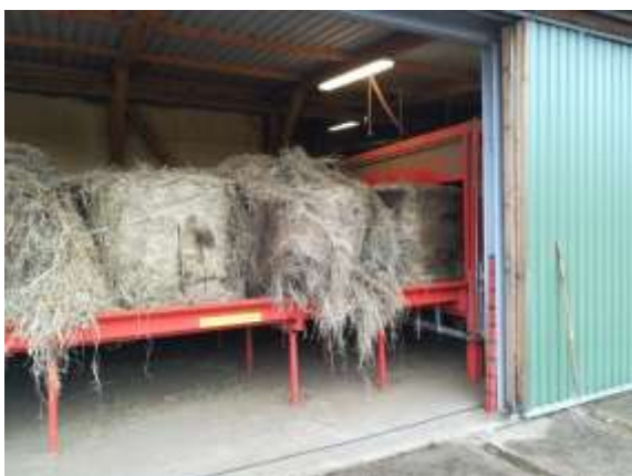
Bales of sedge lying on the conveyor in front of the round bale disintegration unit (Photo: Guy Kabengele)
