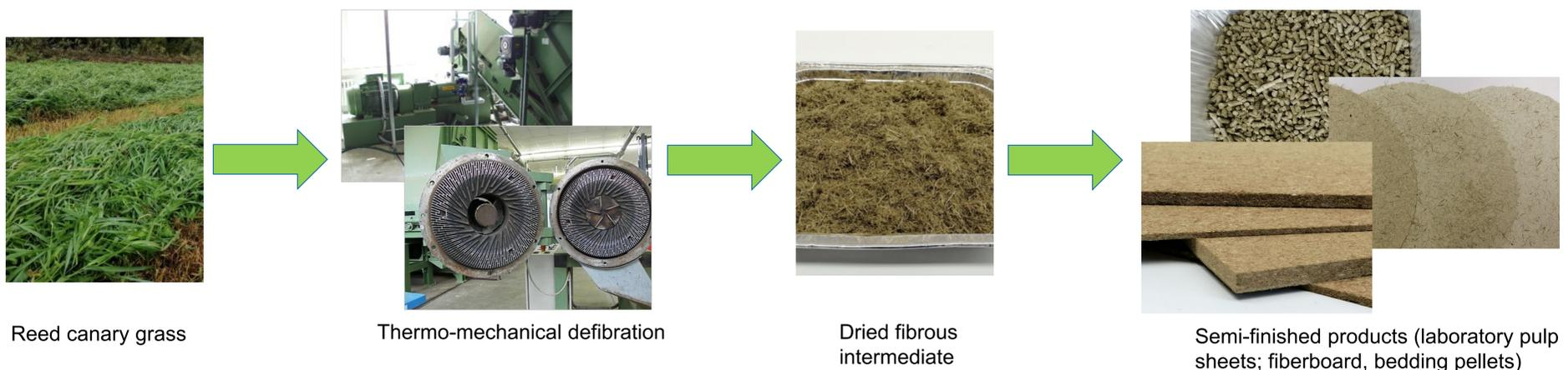
First processing trials with wet paludi-biomass such as reed canary grass in a thermo-mechanical process (defibration extruder + disk mill) resulted in a promising pulp. In dried form, this prepared raw material could be processed into first semi-finished products with promising properties. Possible applications in the pulp molding sector, in the bedding market of organic agriculture and as fiber material boards are just a few examples of the utilization potential of paludi-biomass in future.
