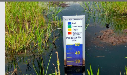
Water level marker to monitor ground water level.
