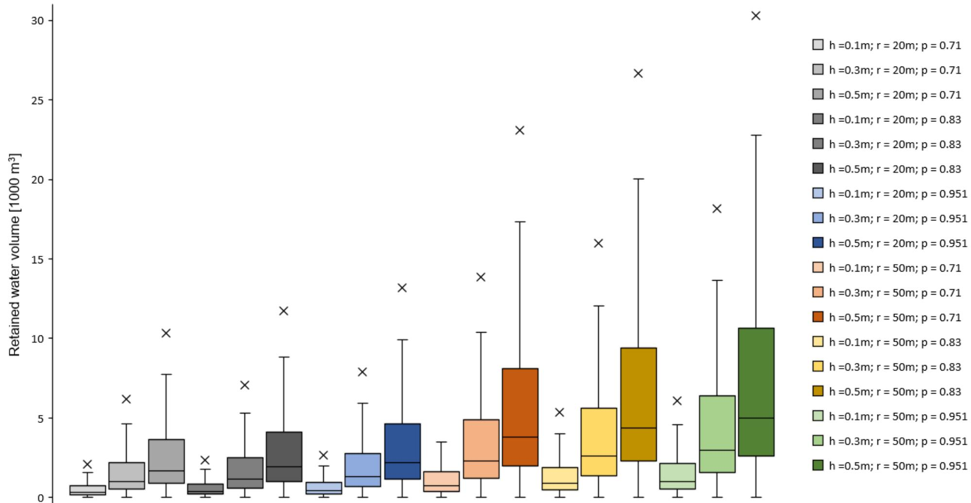
Fig. 1. Boxplots comparing retained water volume in 18 scenarios, using various values of the average radius of water level rise in a cross-sectional view from the ditch, porosity and stacking height (outliers excluded).
